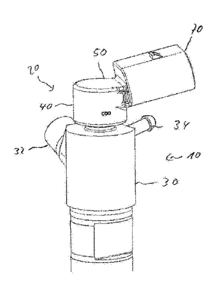
predefined position. The cover may close a cavity defined by the housing unit and be coupled mechanically to the housing unit. The first sealing element may be arranged between the housing unit and the cover to prevent penetration of solid, liquid, or gaseous media into the cavity.
