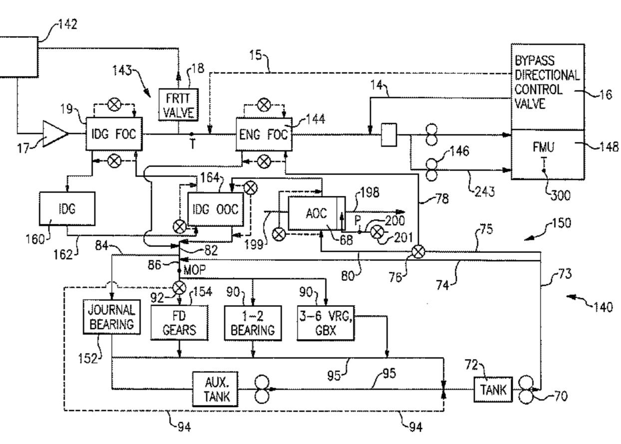
line directed through one or more heat exchangers at which lubricant is cooled. The cool line then is routed to a fan drive gear system of an associated gas turbine engine. A method and apparatus are disclosed. The heat exchangers include at least an air/oil cooler wherein air is pulled across the air/oil cooler to cool oil. The air/oil cooler is provided with an ejector tapping compressed air from a compressor section to increase airflow across the air/oil cooler.
