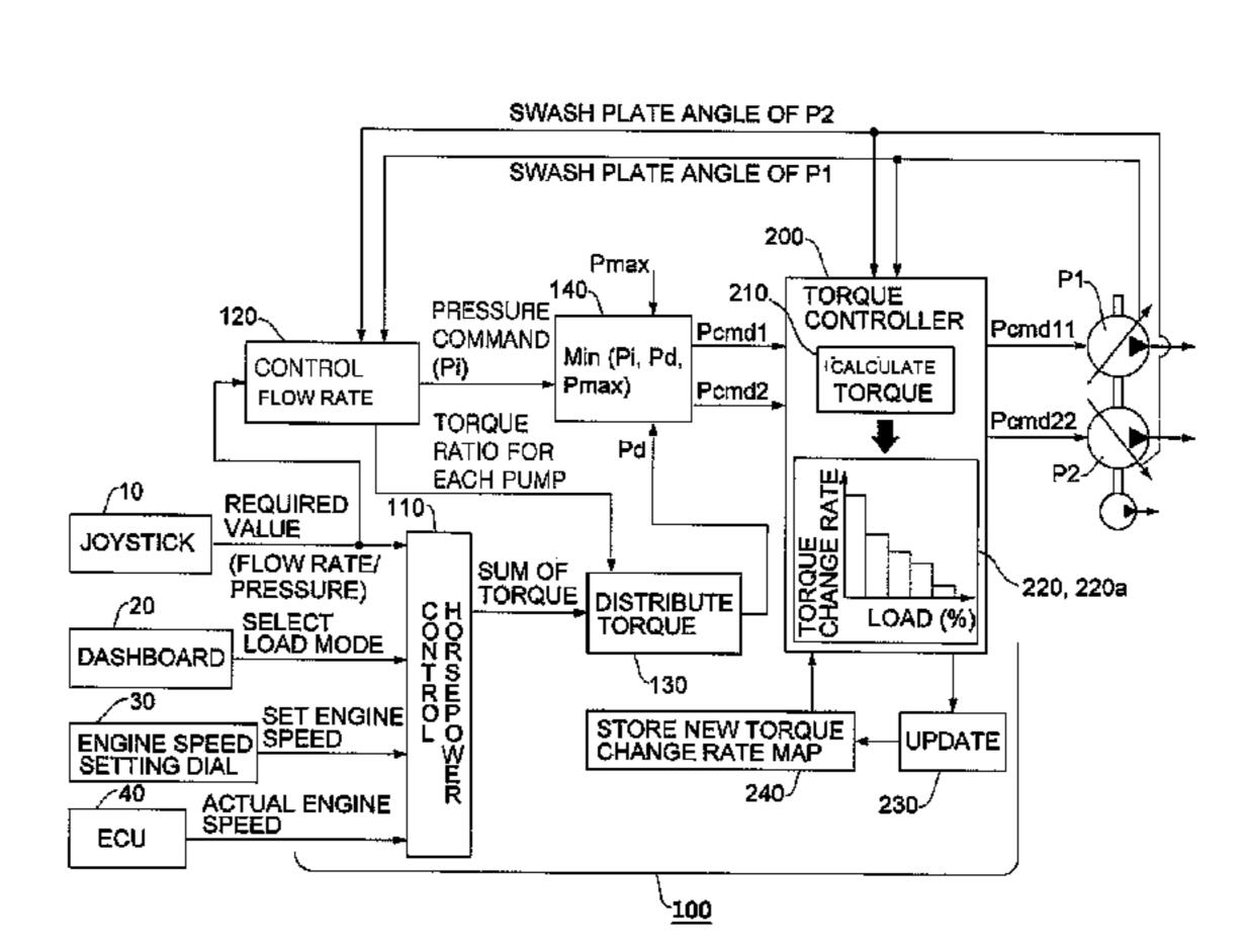
generating a torque change rate for each load section based on the information collected in the information collecting step; and updating an existing torque change rate map to the new torque change rate map generated in the map data generating step.
