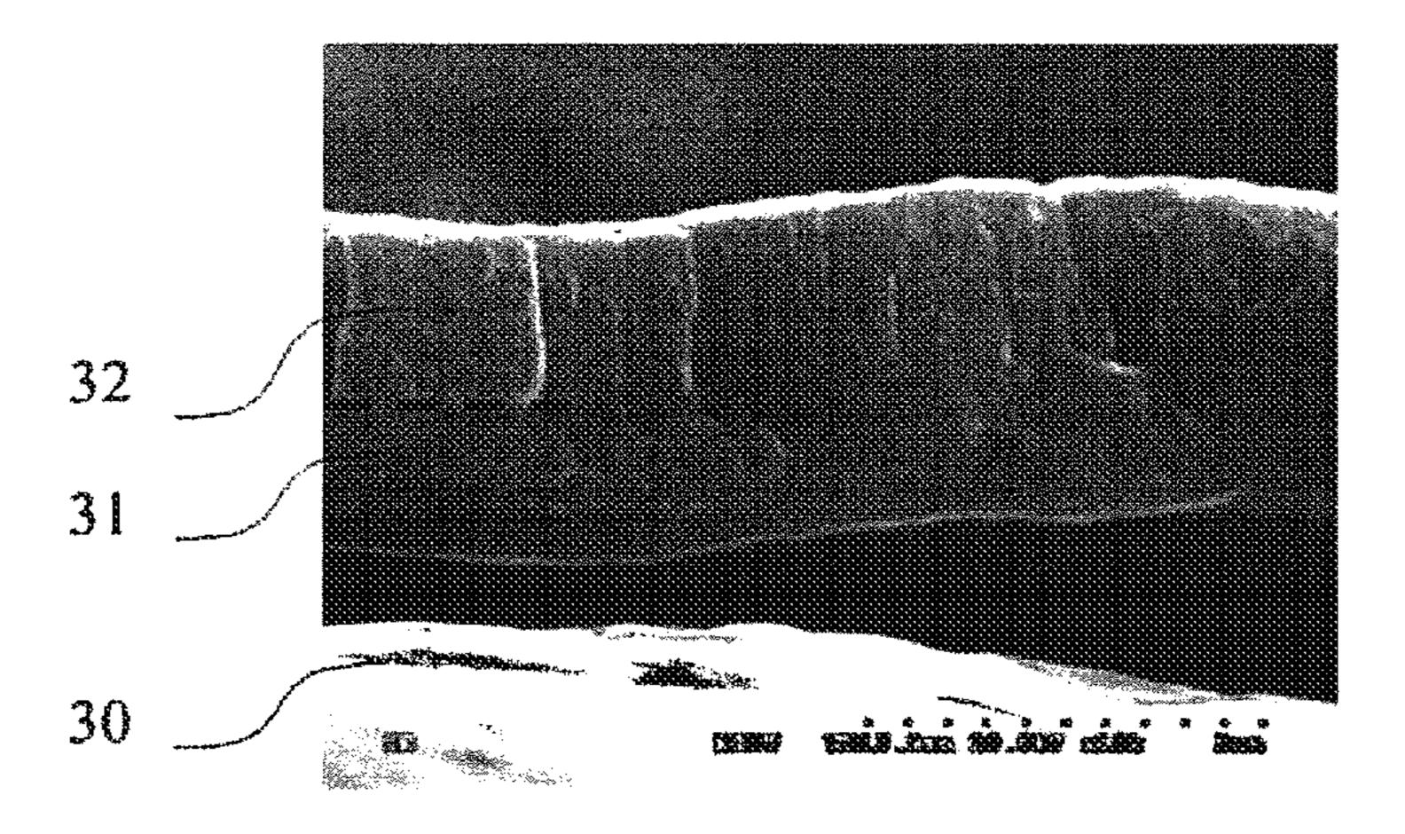
aluminum alloy layer formed on a top surface of the steel sheet and a second magnesium-aluminum alloy layer formed on a top surface of the first magnesium-aluminum alloy layer, wherein a magnesium content of the first magnesiumaluminum alloy layer is higher than that of the second magnesium-aluminum alloy layer.
