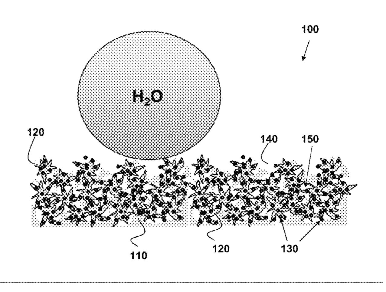
that if the surface is damaged during use, freshly exposed surface will expose a coating identical to that which was removed, for extended lifetime.
