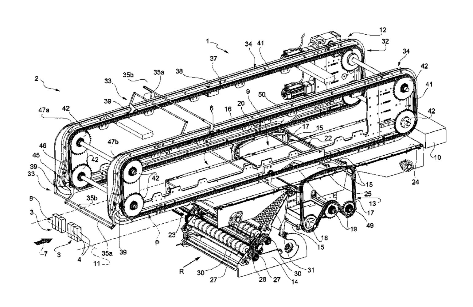
prising a stability control group (12) for preventing said products (3) from tipping along said conveyor (6), said stability control group (12) comprising a plurality of anti-tip devices (33), each of said anti-tip devices (33) being associated, during operation, with a respective product (3) to move together with said respective product (3) through said wrapping station (9).
