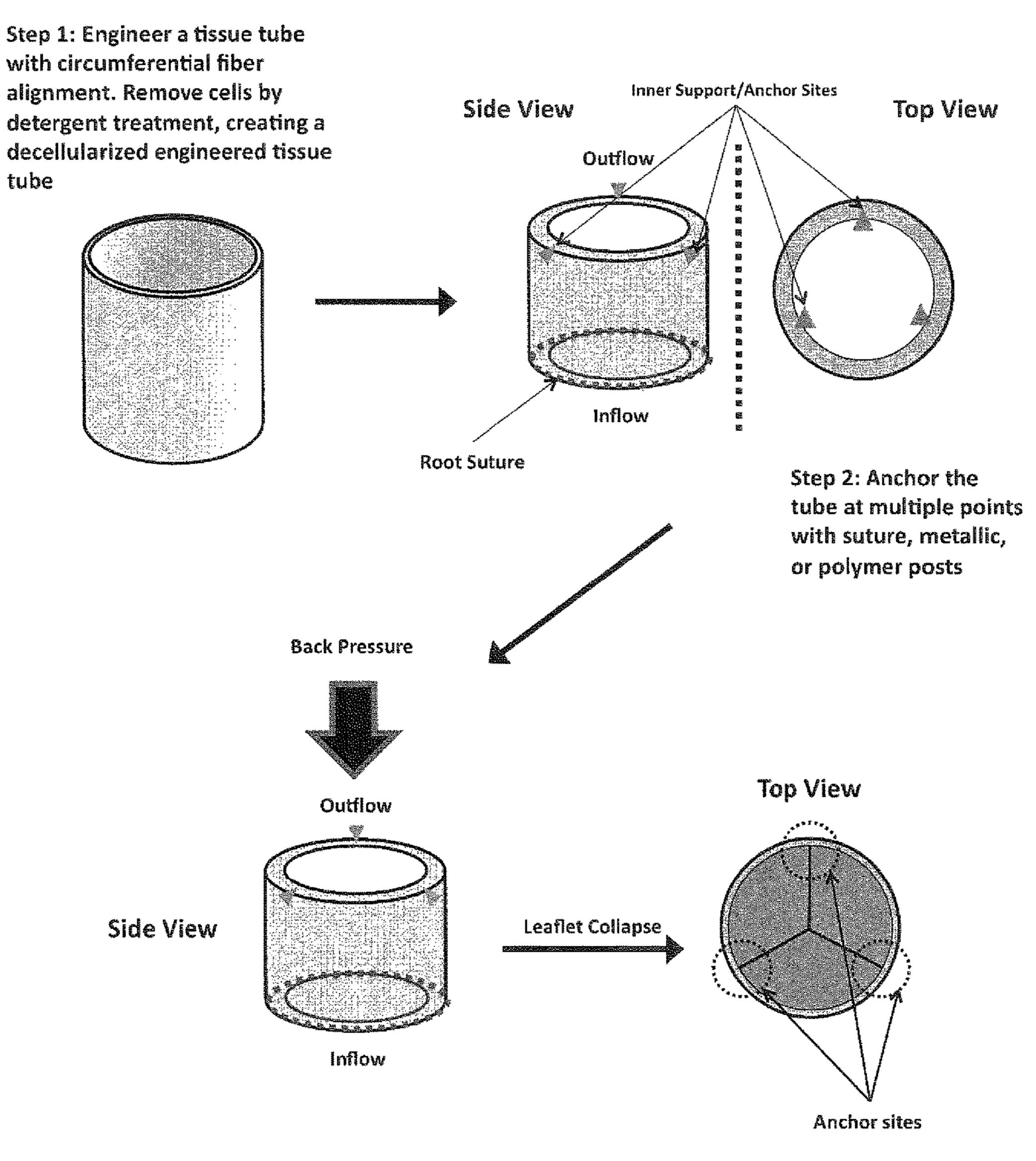
Step 3: With flow, the tube drops inward creating leaflets with functional valve action
