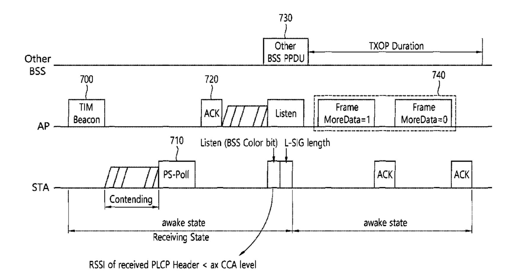
whether or not to switch to a doze state from an awake state on the basis of the reception strength of the different BSS PPDU.
