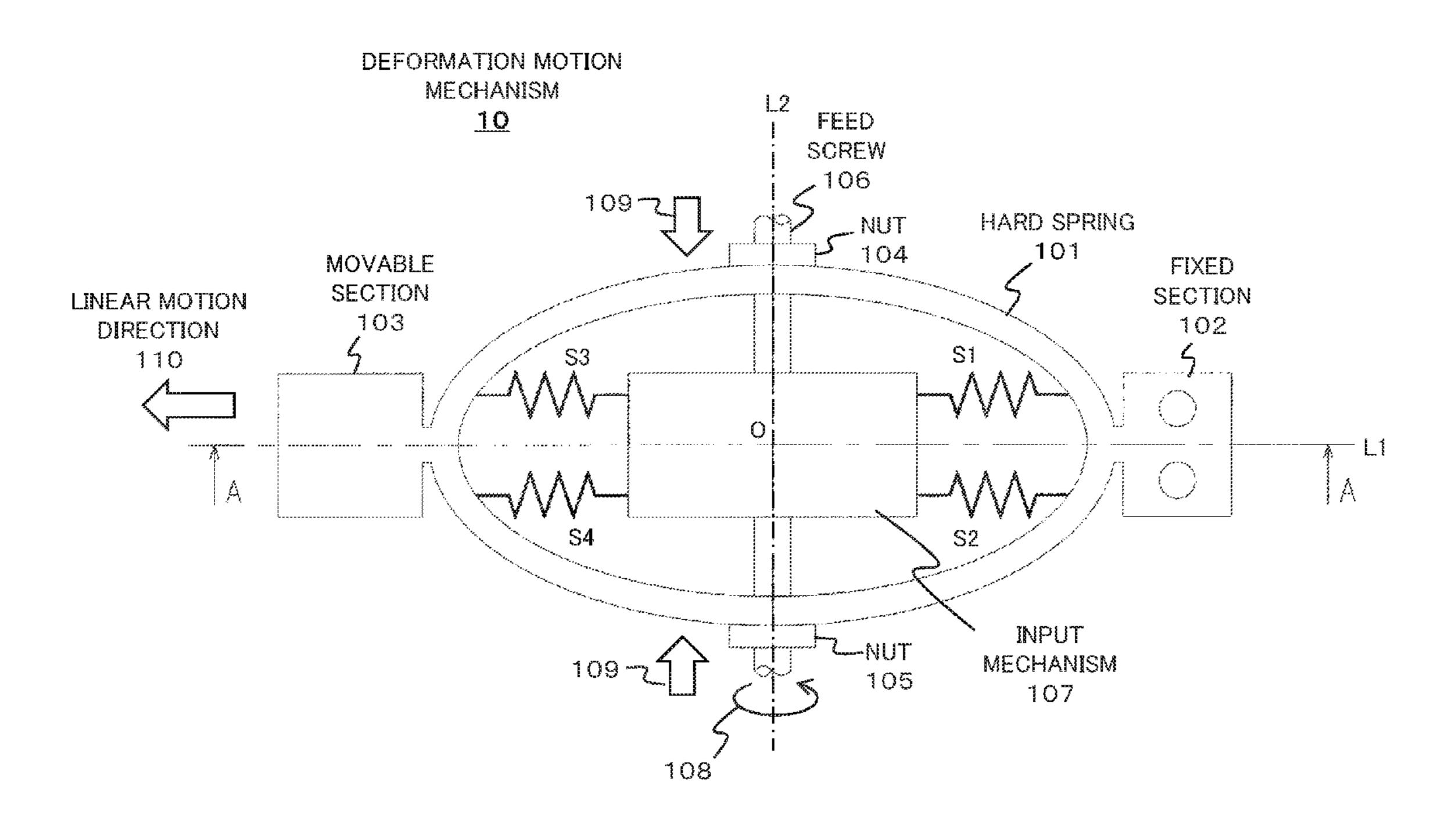
other end is movable along the center line; a drive unit which is placed within the elastic ring member and is arranged to rotate a feed screw engaged with both ends of the elastic ring member along an operating line orthogonal to the center line, to press or stretch the elastic ring member along the center line; and a plurality of flexible arms which connects the drive unit to the elastic member in at least a direction of the center line.
