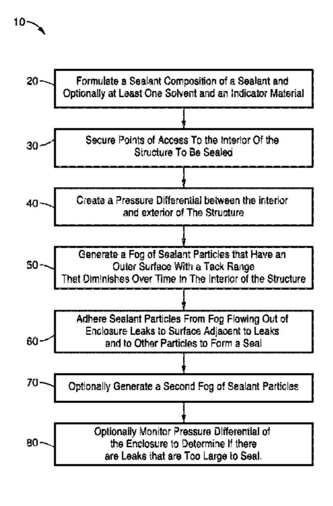
time in the building interior allows control over the treatment area so that leaks are sealed without leaving a tacky residue.
