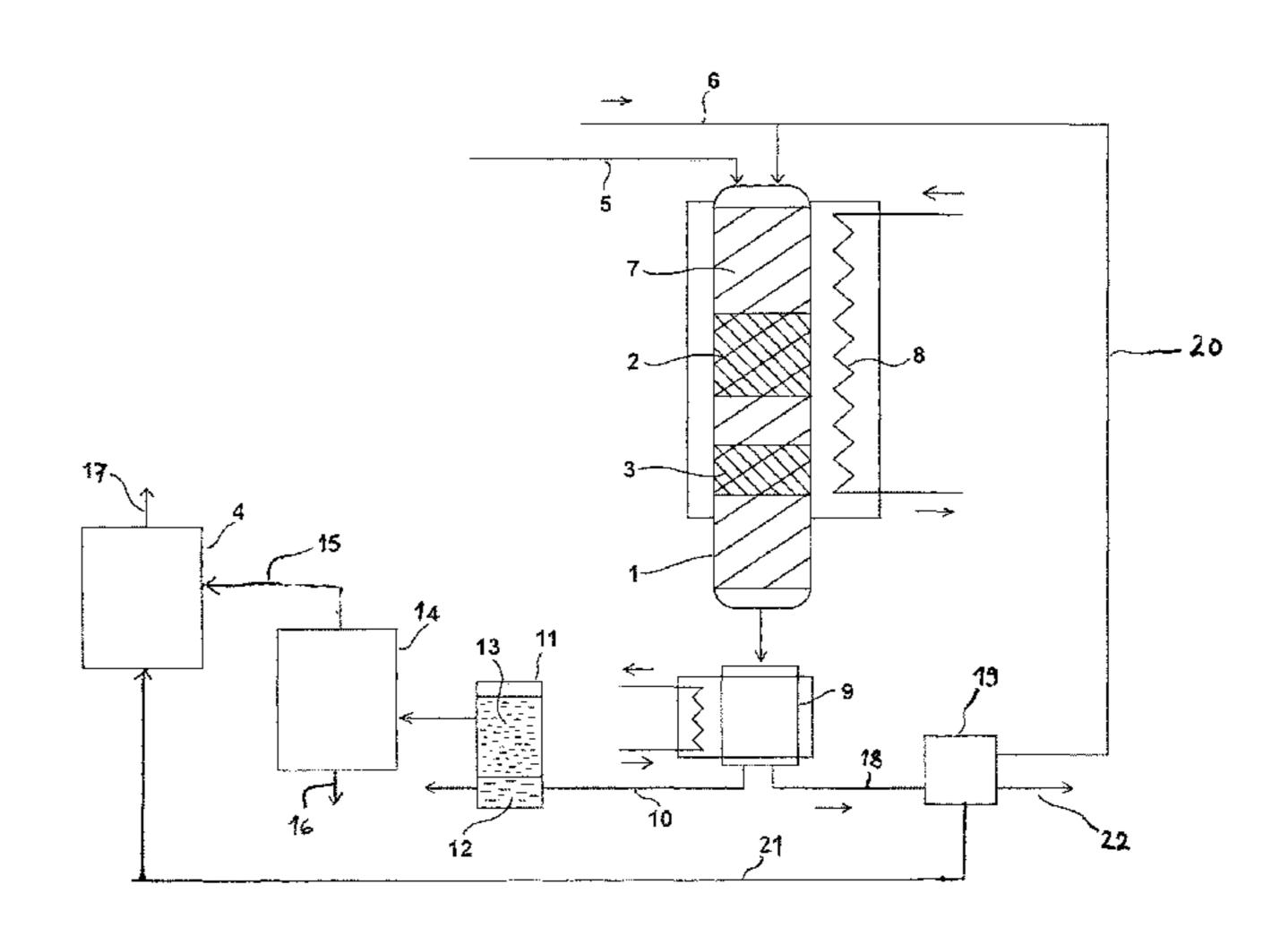
for removal of useless aromatic hydrocarbons and then to steam cracking to form a product containing olefins such as ethylene or propylene. By regulation of the deoxygenation temperature to be at least 270° C. but less than 360° C. the yield is rich in linear and cyclic aliphates that usefully turn to olefins in the steam cracking, while formation of napthalenes is reduced.
