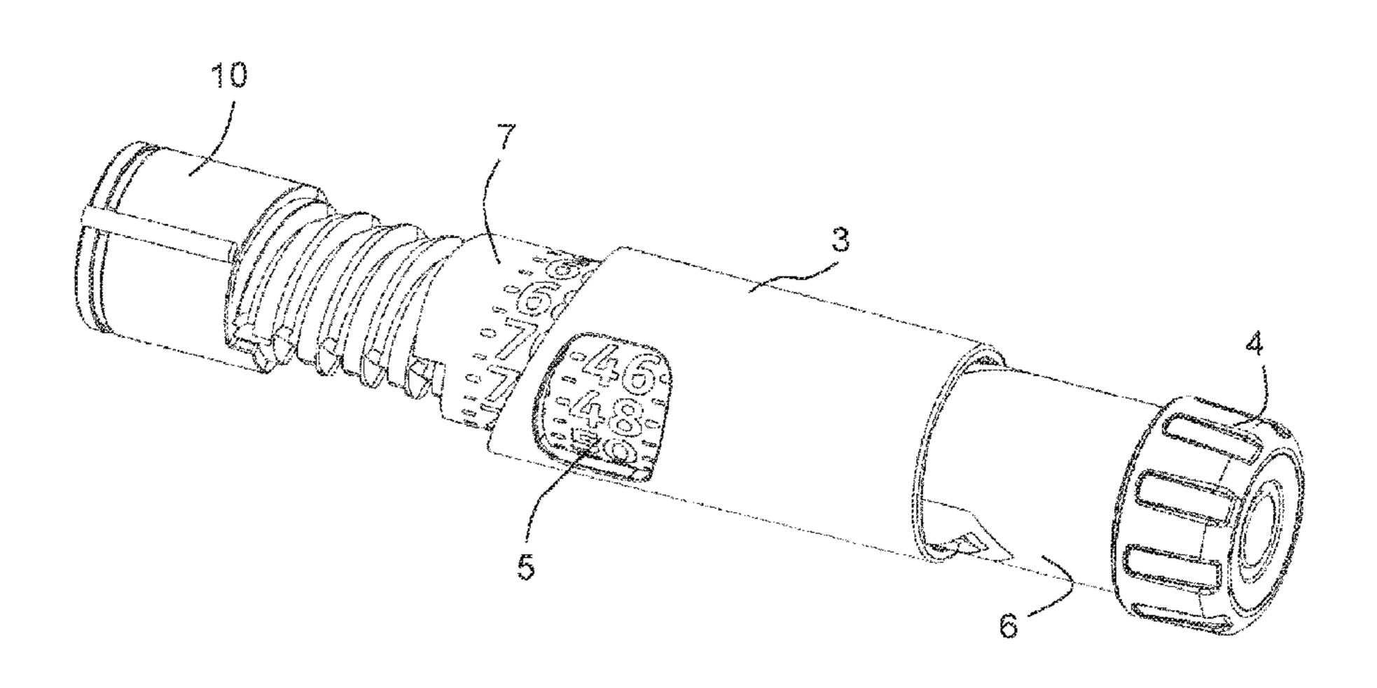
primed state of the assembly, with the first sleeve member being in the second position relative to the second sleeve member, first and second sleeve members are permanently rotationally and axially locked to each other by a first engagement feature such that first and second sleeve members together form a sleeve.
