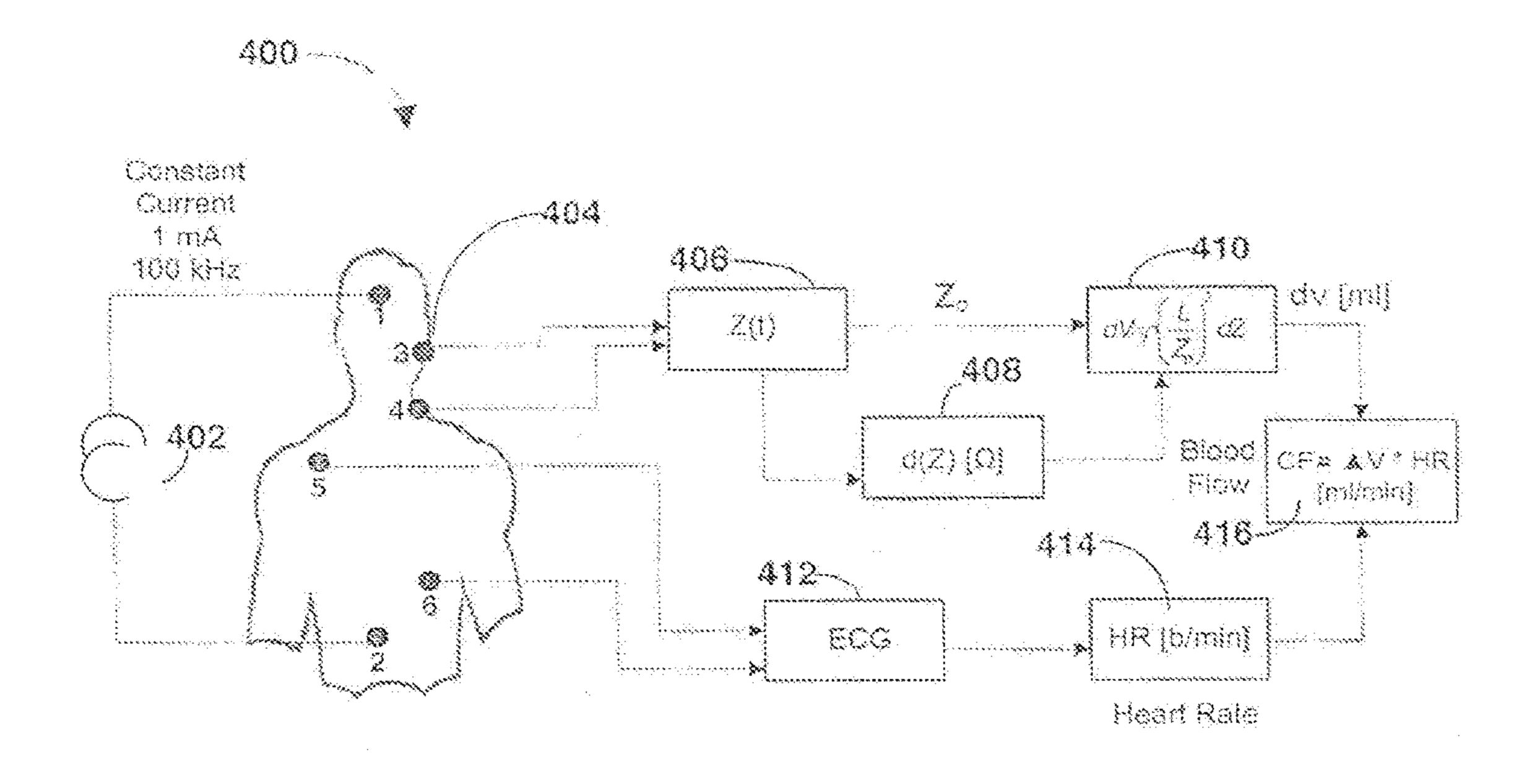
Key: 1 and 2: Current Electrodes 3 and 4: Measurement (voltage) Electrodes 5 and 6: ECG Electrodes
