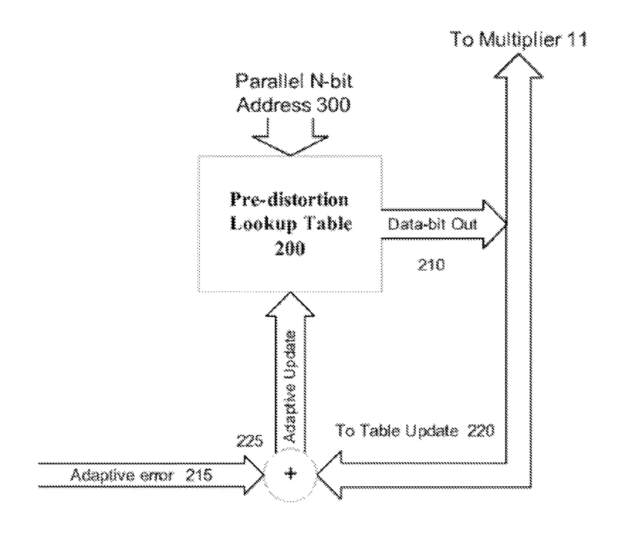
FIGURE 3 The combined time-delay lookup table for predistortion and time-delay compensation using parallel addressing
