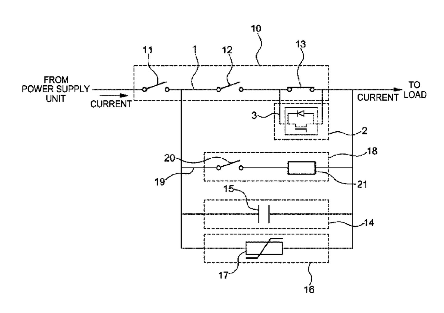
among the high-speed mechanical switches installed in the main conduction unit for current breaking of the main conduction unit; a capacitor installed on a circuit connected in parallel to the main conduction path; and a surge arrester installed to be connected in parallel to the capacitor connected in parallel to the main conduction path. The DC current breaking method uses the DC current breaker.
