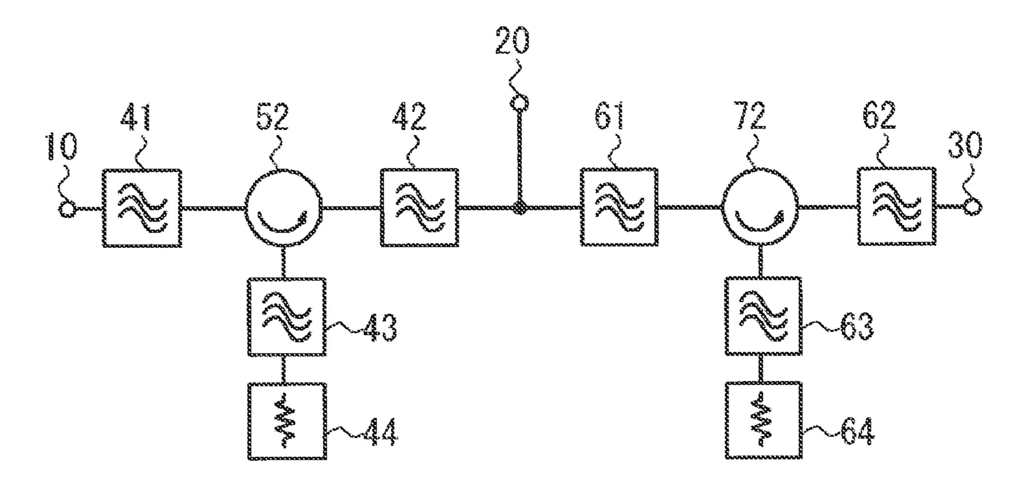
provided in a stage subsequent to the first reception-side filter. The reception-side directional propagation circuit is connected between the first reception-side filter and the second reception-side filter.
