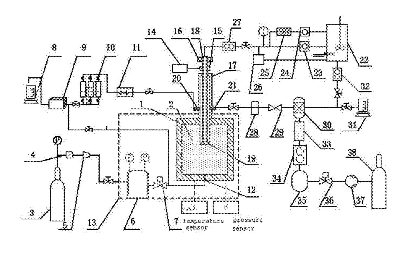
formation drilling process, a hydrate exploitation process and a produced gas collecting and processing process. With this simulation device and method, the external environment can be truly simulated, so that the authenticity and accuracy are better, and the entire natural gas hydrate exploitation process is continuously simulated and comprehensively evaluated to provide guidance for natural gas hydrate exploitation.
