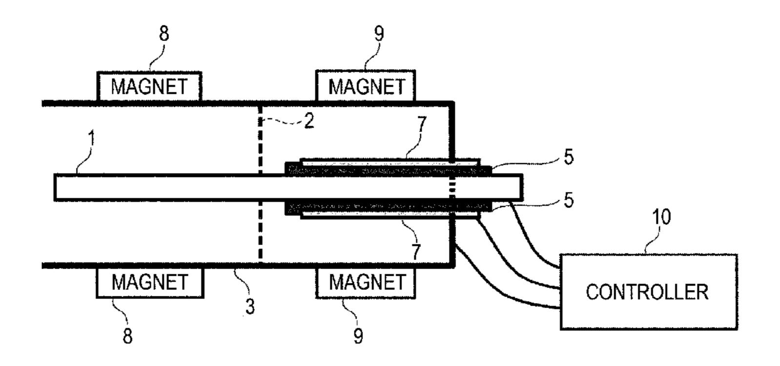
operation mode and a contamination diagnosis mode, the cold cathode ionization vacuum gauge comprising: an anode 1 and a cathode 3 that are for measuring vacuum pressure in the normal operation mode; an anode 7 and the cathode 3 that are for measuring the vacuum pressure in the contamination diagnosis mode; and a controller 10 that compares the size of a current measured between the anode 7 and the cathode 3 and the size of a current measured between the anode 1 and the cathode 3.
