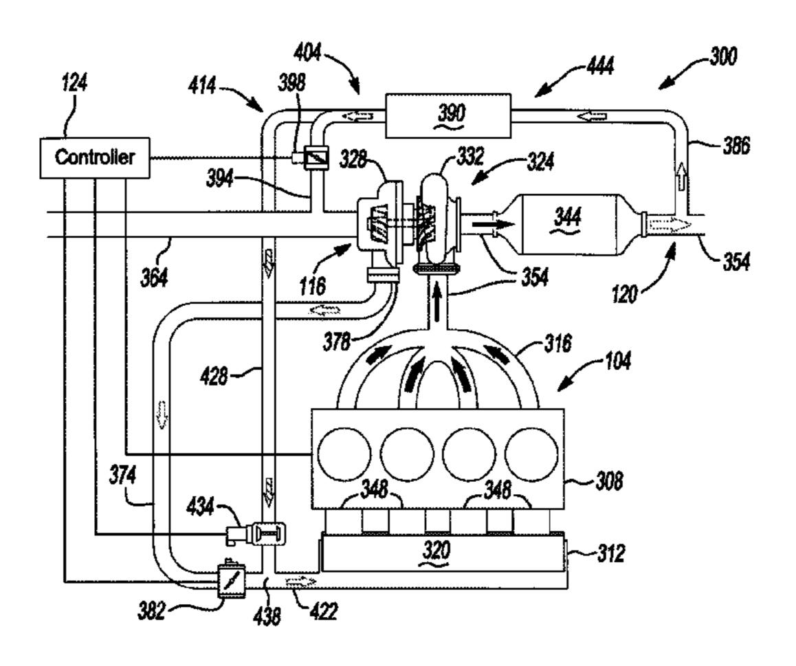
operating conditions thereby providing EGR directly to the intake system that bypasses the turbocharger and throttle valve.
