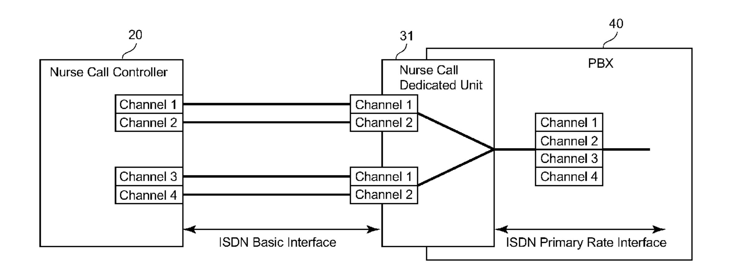
a private branch exchange serving the mobile terminals have been connected to each other through a nurse call adaptor; thus, there is a need for one such nurse call system that does not require a nurse call adaptor. Provided is an interface unit which is connected to a nurse call controller through a plurality of ISND basic interfaces, connected to a private branch exchange through an ISDN primary rate interface, and performs interface conversion therebetween.
