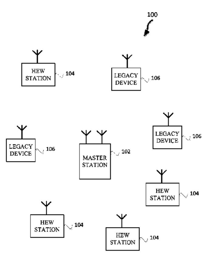
bols, and transmit the longer-duration OFDM symbols on channel resources in accordance with an orthogonal frequency division multiple access (OFDMA) technique. The channel resources may be resource allocations with each resource allocation including the one of the predetermined number of data subcarriers.
