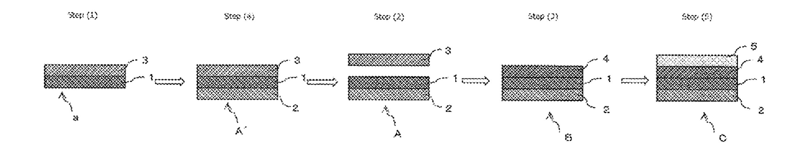
wherein the liquid material contains a resin component or a curable component capable of forming a resin layer. This production method enables the achievement of a polarizing film which is able to have satisfactory durability in a heated environment even in cases where a thin polarizer is used therefor.
