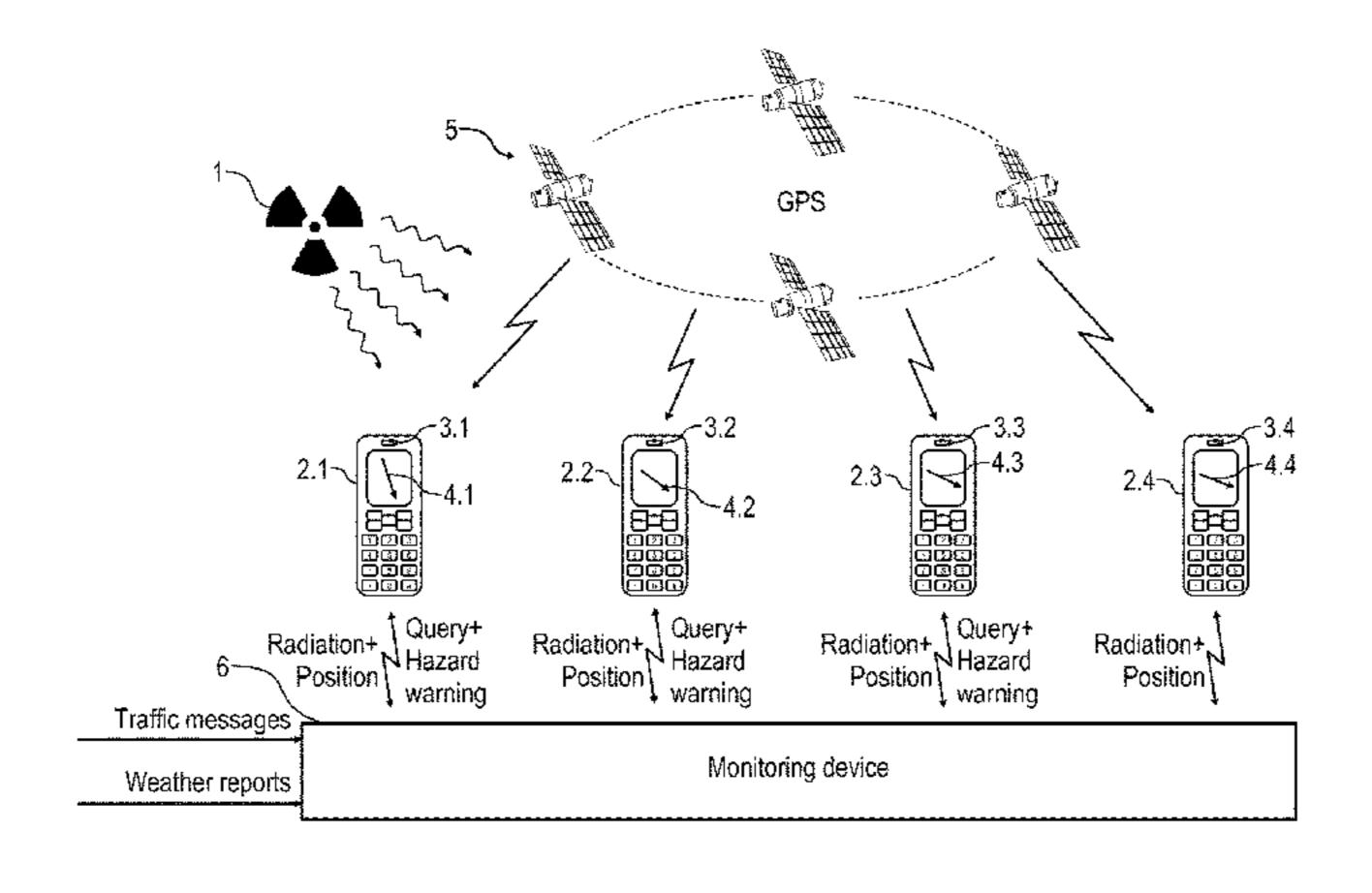
plurality of spatially distributed electronic terminals (2.1-2.4), in particular from mobile telephones with an image sensor for measuring the radioactive radiation. The invention further relates to a corresponding terminal (2.1-2.4) and to a complete monitoring system with a monitoring device and numerous terminals (2.1-2.4) for measuring the environmental variable.
