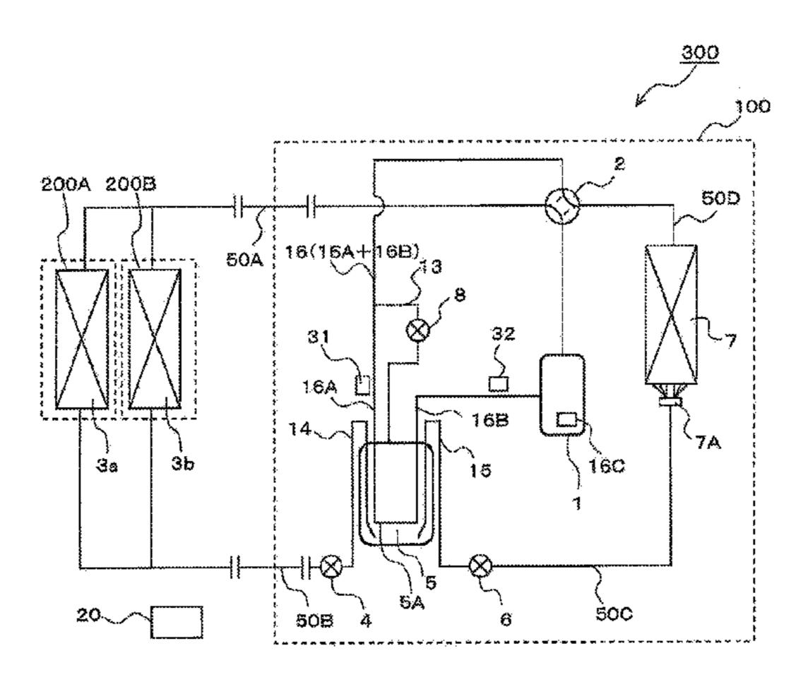
configured to control an opening degree of the flow control valve based on a degree of superheat of refrigerant in the heat recovery portion.
