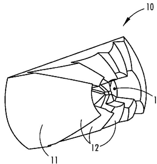
shaping the incident light into a collimated light pattern emanating from the exit surface. Further, the plurality of optical elements may be configured in a step-wise pattern defined by a sweep angle.
