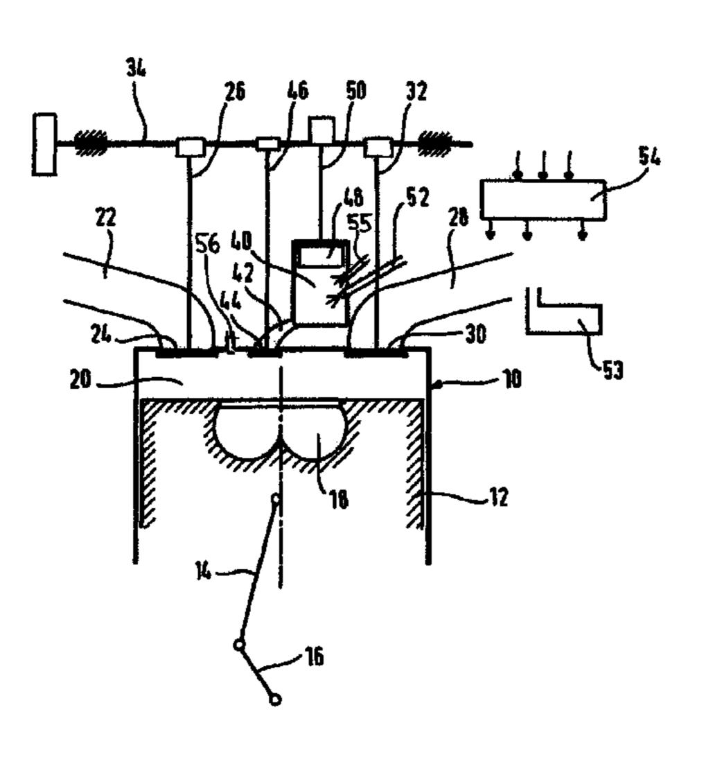
fresh air from the power chamber goes into the ancillary chamber and such that fuel is expelled from the ancillary chamber into the power chamber via the flow-through valve for combustion with fresh air compressed in the power chamber.
