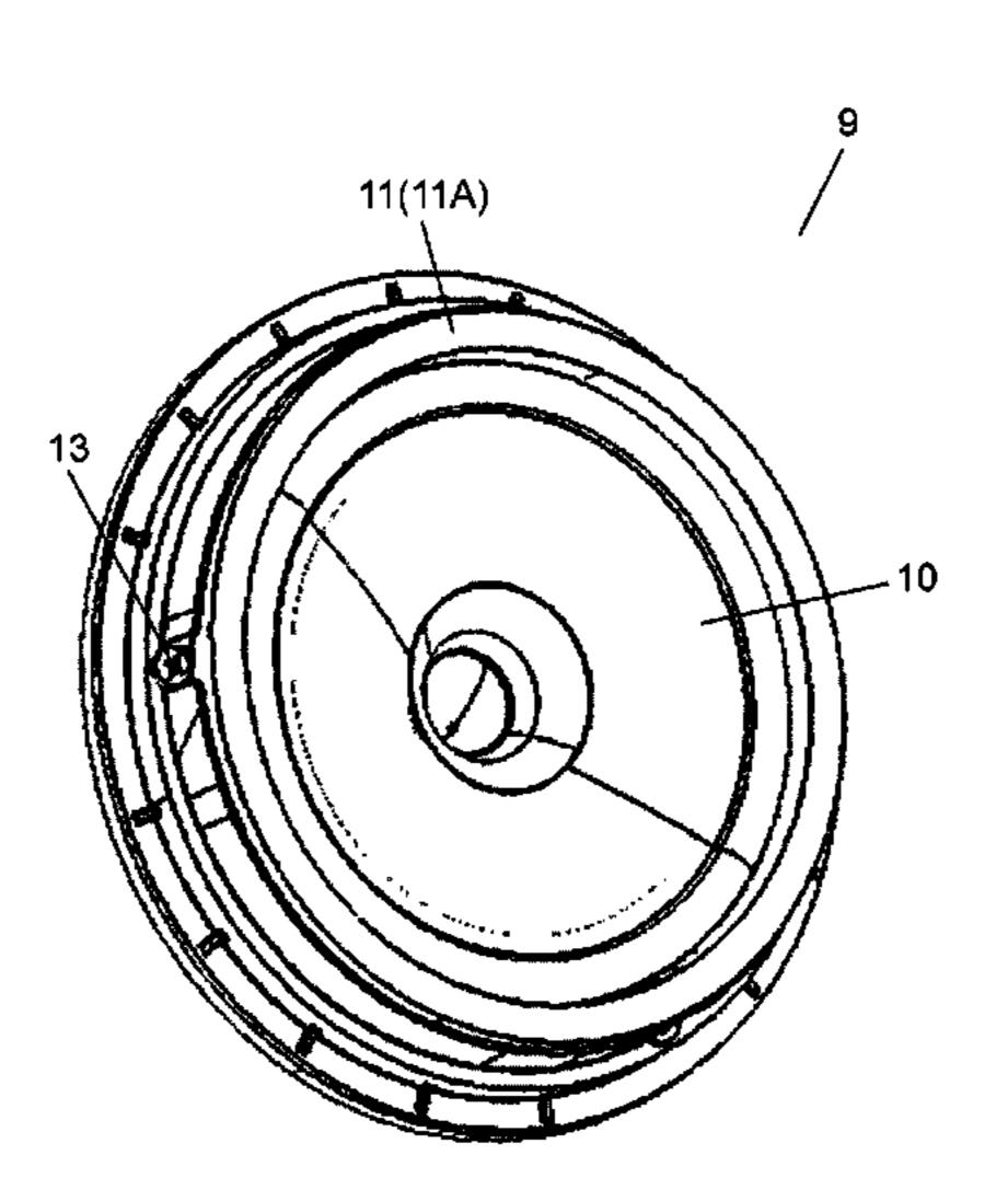
surface; and a locking portion disposed on a side near the bottom surface of the base portion. The fixing member penetrates the frame from the front surface to the mounting surface and is fixed to the base portion by screwing.
