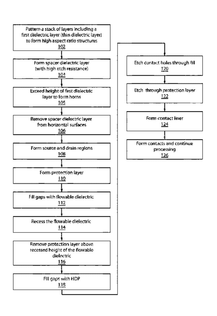
the etching processes. The gaps are filled by a high density plasma fill.
