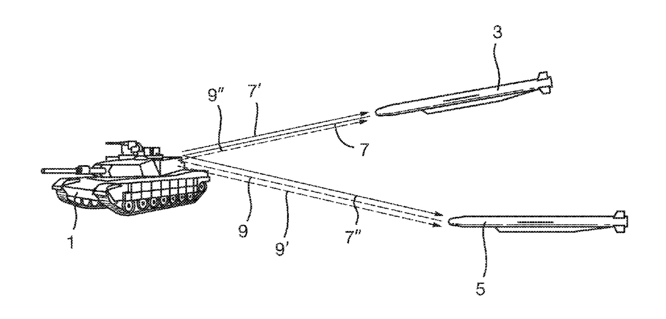
may enable the designator to perform other tasks, while the missile tracks and engages the target.
