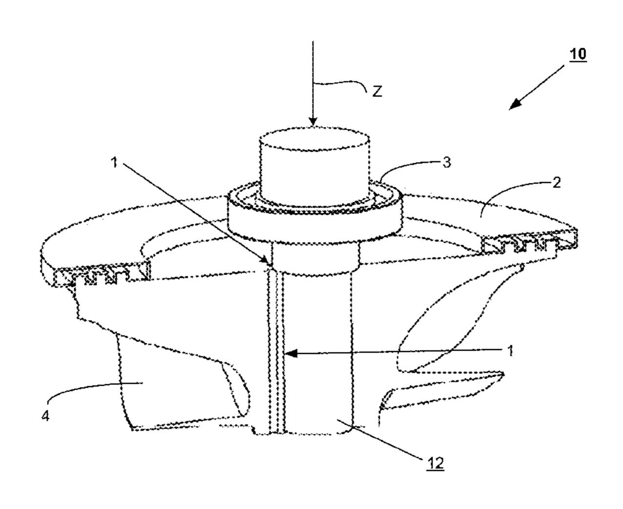
sionless speed of about 0.7 and a loading coefficient of 0.7 is a preferred expansion machine for certain thermodynamic cycles involving CO2 gas to permit such radial turbines to operate close to their optimum design specification and highest efficiency level. Methods to handle liquids which may condense within or inside the turbine are also disclosed, as well as methods to handle axial pressure on bearings and methods to protect lubricant in bearings.
