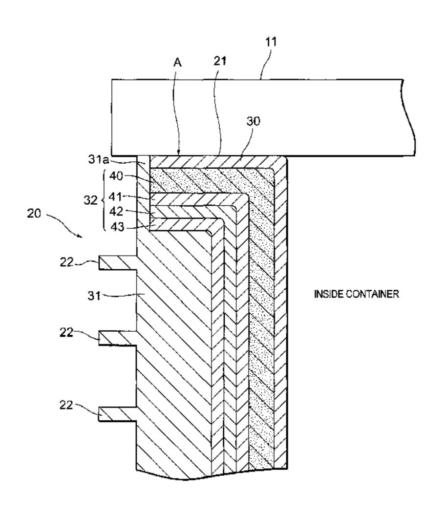
forms the upper end surface of the opening part. When the sealing member is unsealed, part of the innermost layer on the upper end surface of the opening part is configured to be peeled off so as to leave an unsealed mark.
