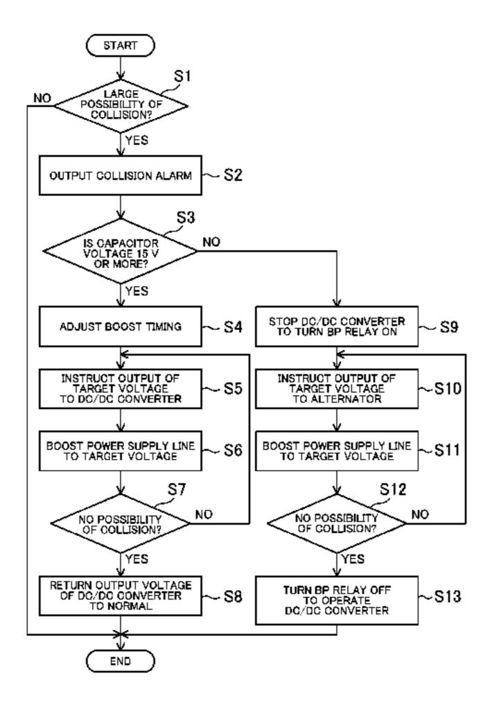
DC/DC converter is set at a target higher than an output voltage in a normal state before brake actuation, or if output of the DC/DC converter cannot be set at the target voltage, the alternator is driven to connect a generation voltage of the alternator to the supply line.
