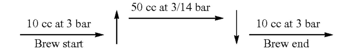
As an alternative, the dispensing or infusion step can occur at a constant pressure comprised between 3 and 14 bar.
