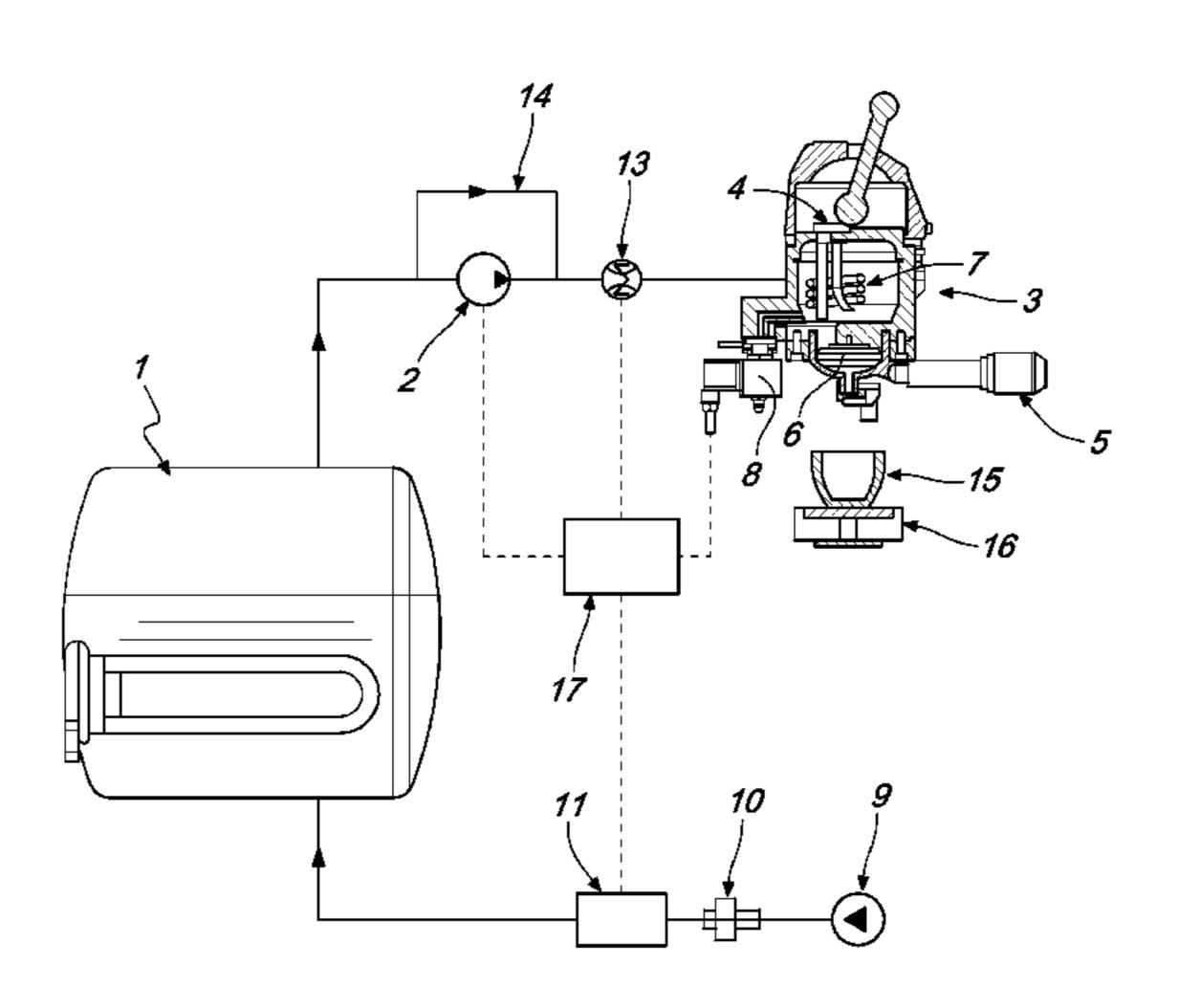
volume is dispensed following calculation of the weight of the ground coffee in the filter and the product dispensed according to a brew ratio.
