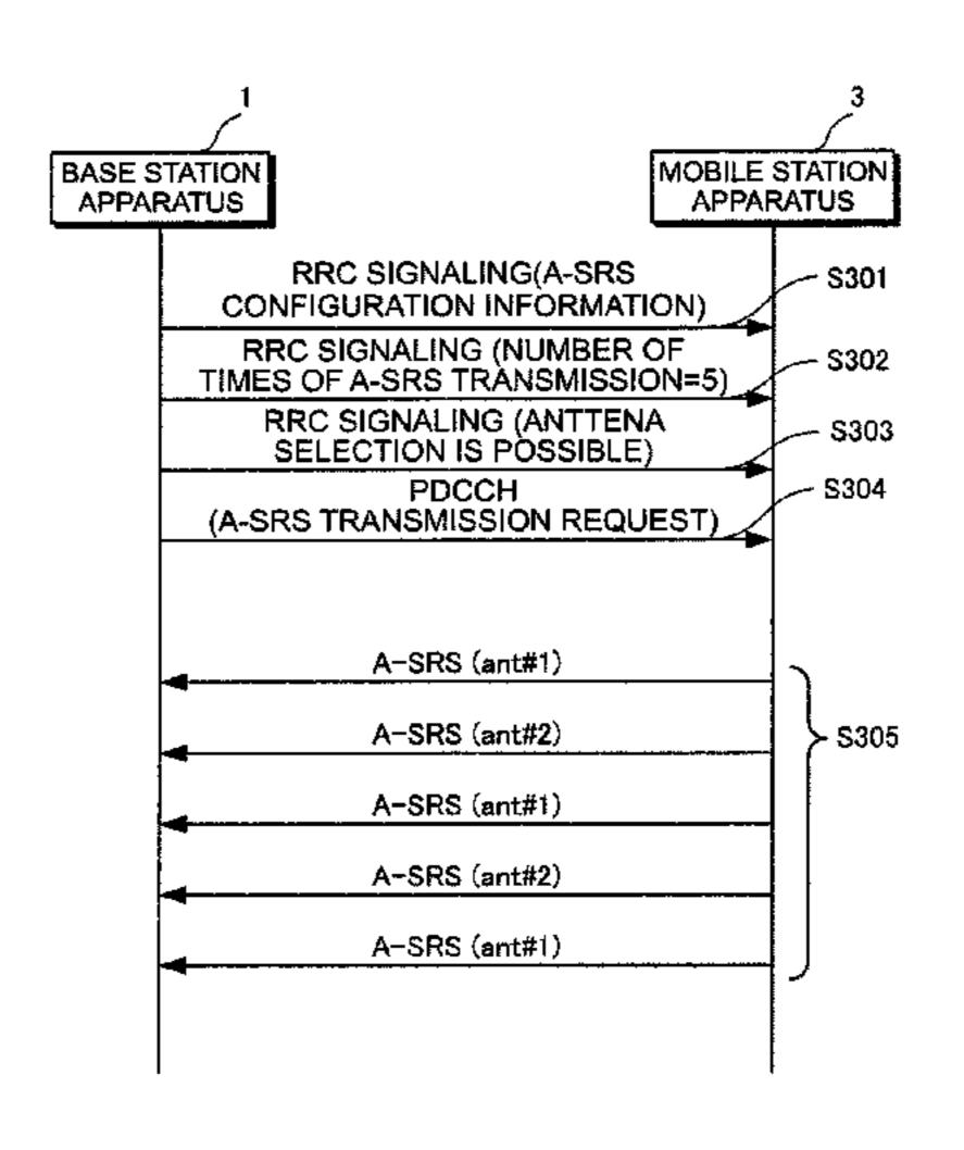
information indicating transmission of the reference signal is included in the physical downlink control channel.
