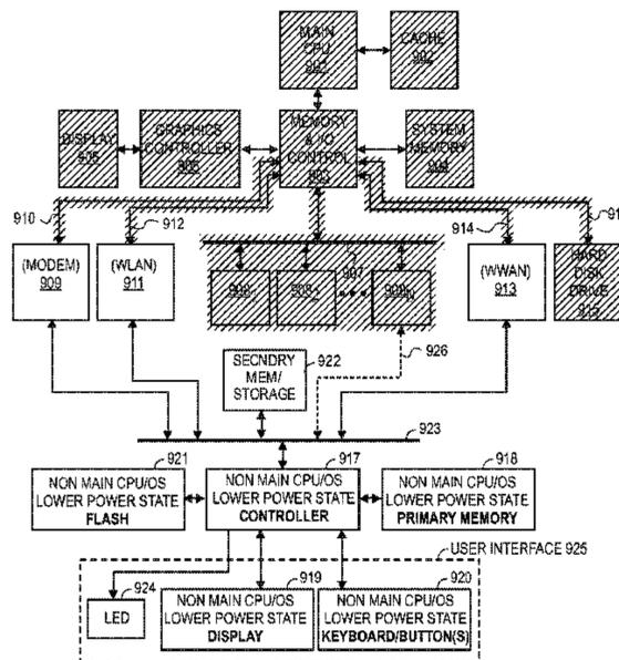
microcontroller and communication between at least some of the plurality of peripheral devices is facilitated using the microcontroller when in an awake state.
