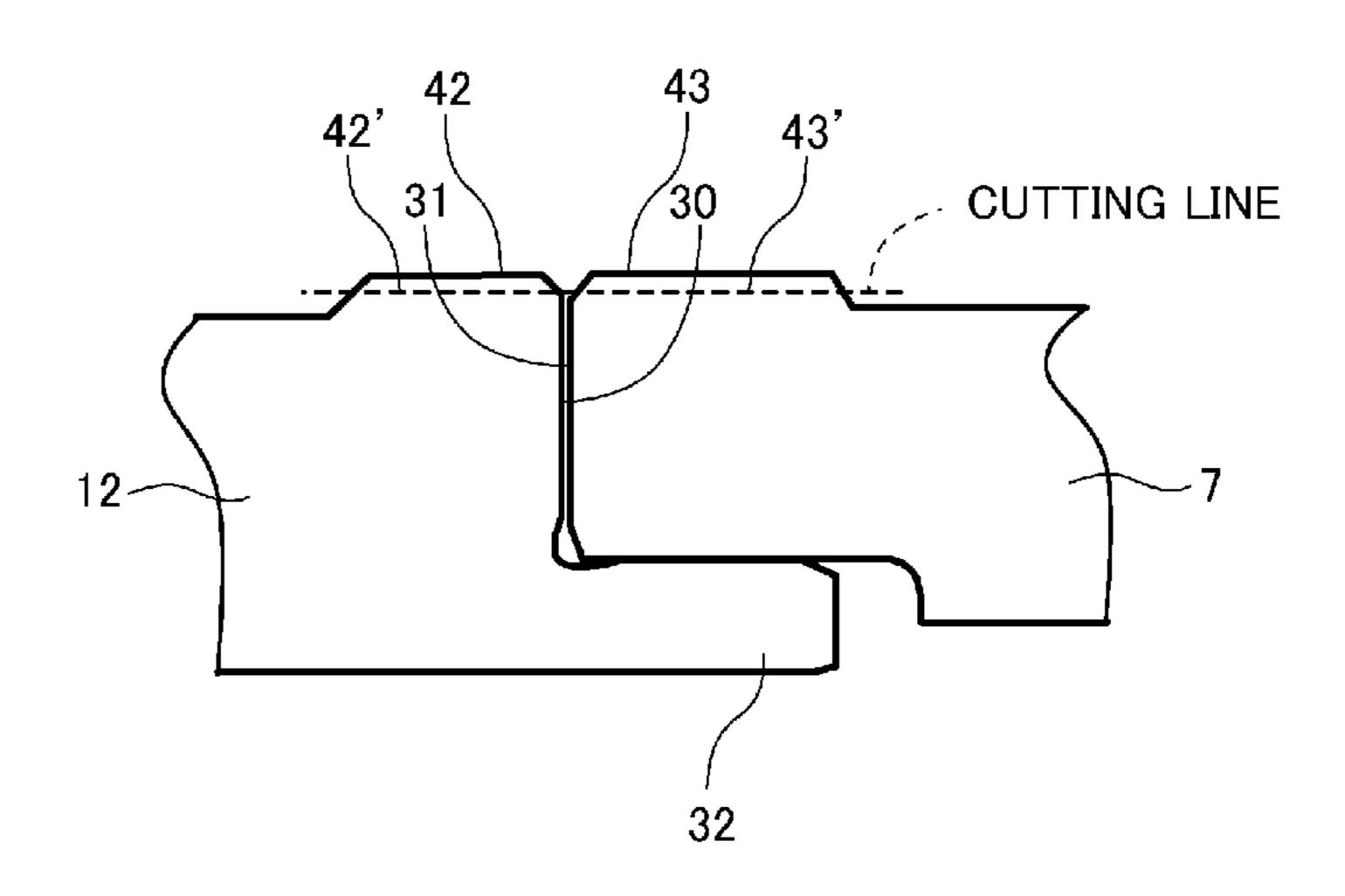
outer peripheral surfaces are equal to each other. With the opening-side end portions abutting against each other, a high-energy beam such as a laser beam (R) is radiated toward the abutment surfaces (30, 31) from the radially outer side to weld the abutment surfaces to each other. Consequently, it is possible to perform welding accurately through easy processing in order to easily manufacture a fluid coupling with high precision that facilitates post-processing.
