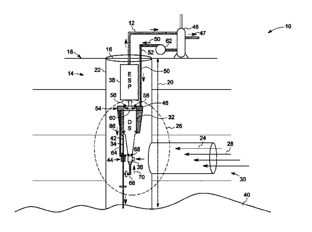
lic motor disposed within the well formation and operatively coupled to the downhole rotary separator, wherein the hydraulic motor is configured to drive the downhole rotary separator using a drive fluid comprising the hydrocarbon rich stream or the second water stream.
