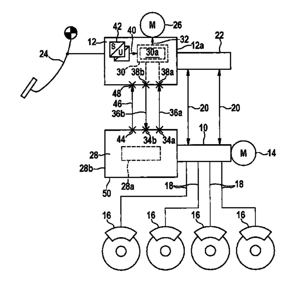
relating to a current actuation of a brake actuating element, and by which a specification signal corresponding to the at least one determined motor target quantity can be outputted to the brake booster control device. The brake booster control device has a second control electronics that, at least in a normal mode, outputs the control signal to the motor of the electromechanical brake booster, taking into account the specification signal outputted by the hydraulic control device.
