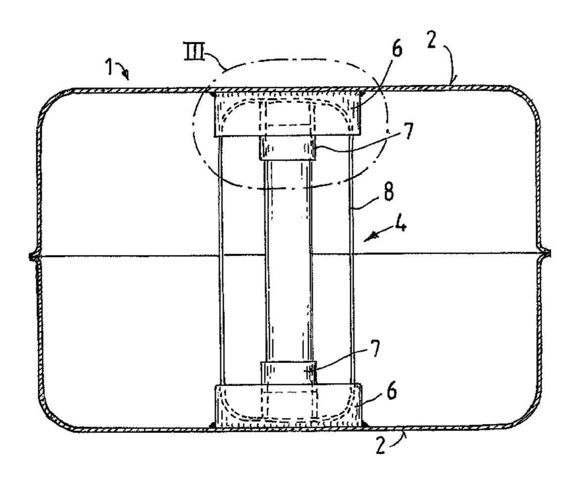
tension-resistant bracing element in the form of a tension-resistant band (8) which extends between the container walls (2).
