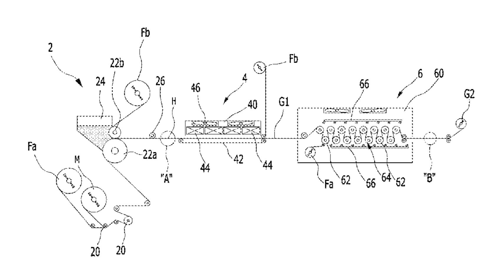
the gel sheet S2. Through the manufacturing method, a gel sheet G2 which is formed to be a film so that density of the front and rear surfaces is higher than a center portion and a beauty pack obtained by pressing the gel sheet S2 by the mask member MP are suggested.
