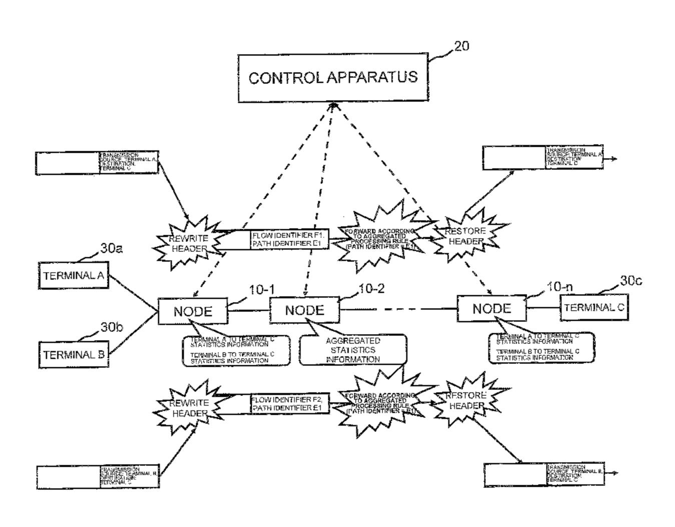
node located intermediate on the aggregatable segment, a common packet handling operation for causing the packet that matches the path identifier to be forwarded according to the packet forwarding path. Then, the control apparatus sets, in a node located at the end point of the aggregatable segment, a packet handling operation for performing restoration and forwarding based on the flow identifier.
