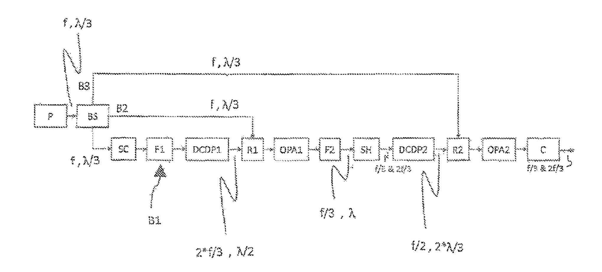
a programmable device making it possible to temporally adjust the pulses corresponding to the bands, in order to allow for the generation of a pulse with a wavelength equal to  $\lambda/3$  and of a duration less than the period of the optical cycle.
