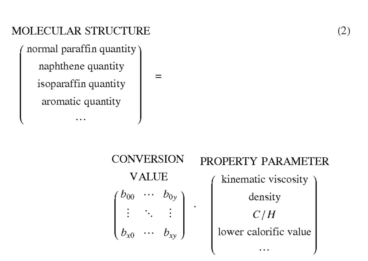
In the formula (2), "b" is a conversion value which is calculated from the sensitivity coefficient "a".
