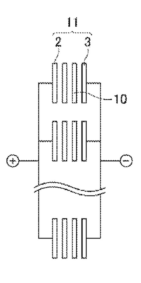
electrolytic cell and heating of the molten salt by a Joule heat generation between a pair of electrodes for electrolysis are simultaneously performed; and wherein the apparatus for molten salt electrolysis has at least two sets of electrode pair, and at least one set of the electrode pairs is electrically opened.
