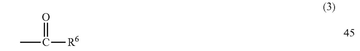
wherein R6 represents a linear or branched alkyl or alkenyl group having from 8 to 22 carbon atoms which may be substituted by a hydroxyl group.
