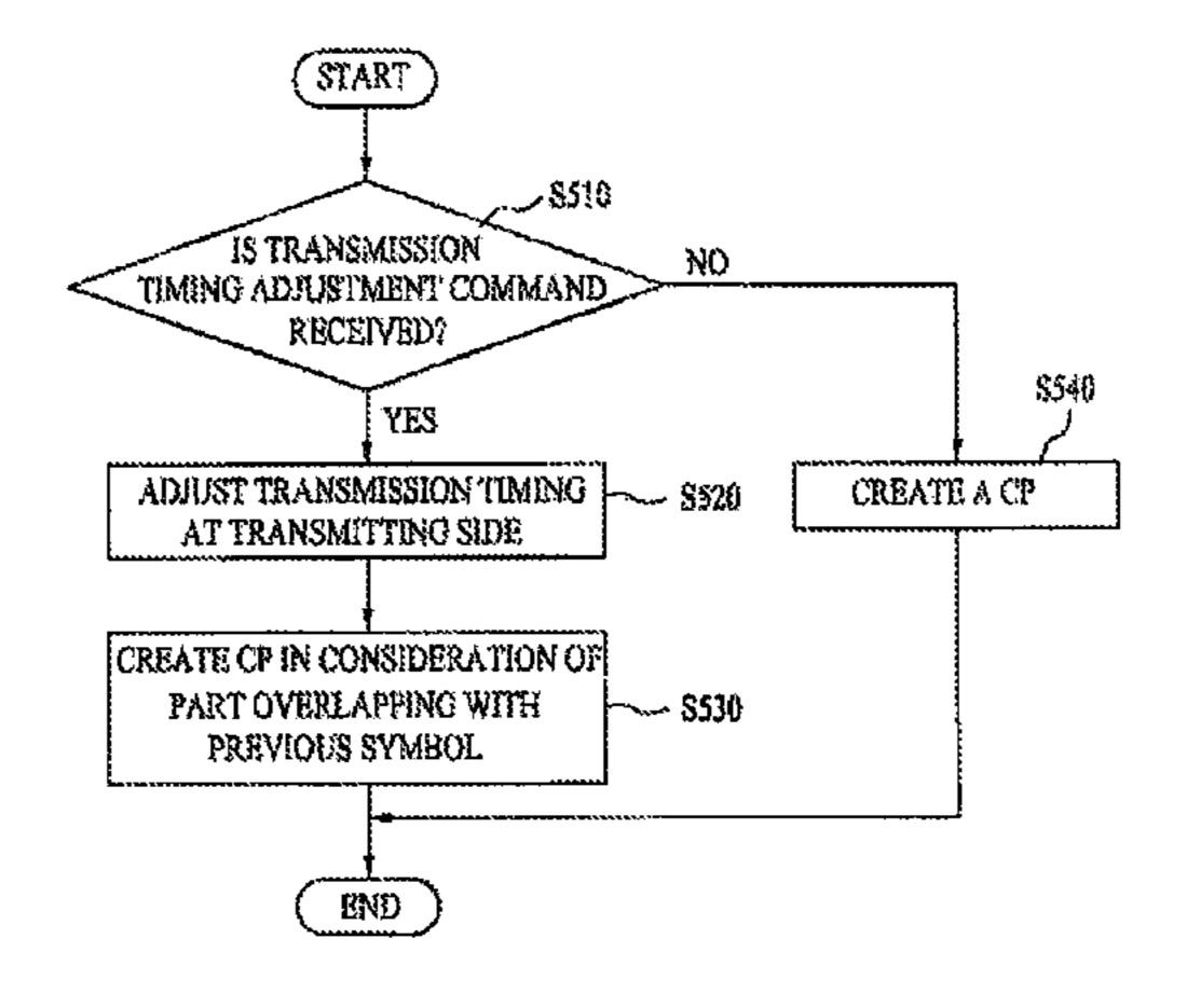
and the second subframe are overlapped, the first subframe is transmitted completely while the second subframe is transmitted partially.
