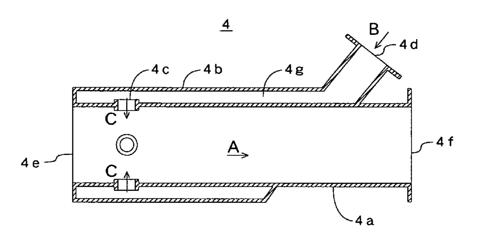
sucking direction. The flow speeds of the low-temperature gas and the high-temperature combustion gas are preferably not less than 40 m/s and not more than 100 m/s.
