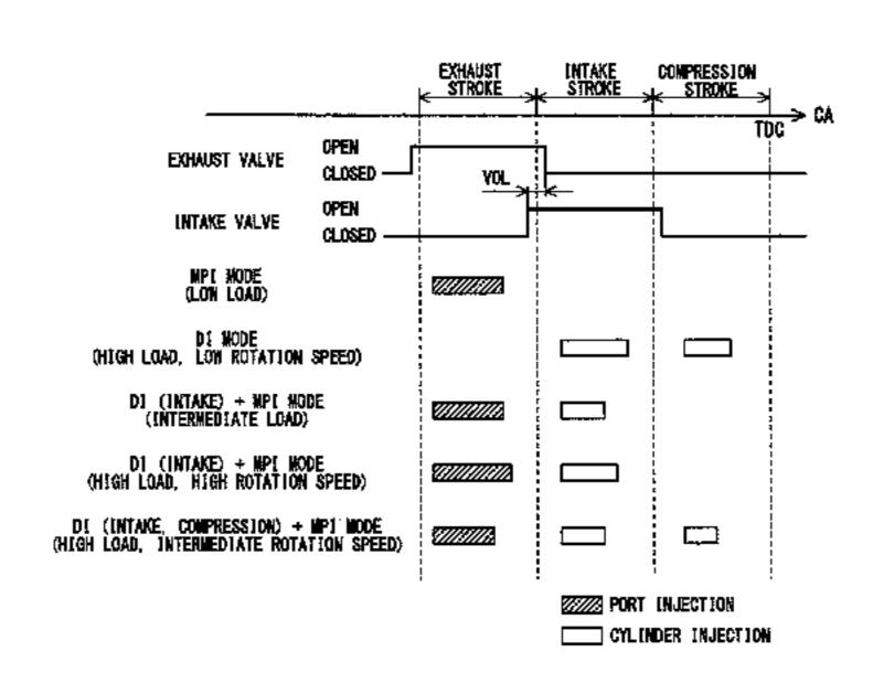
state, causes the fuel to be injected through the cylinder injection valve during an intake stroke, and causes the fuel to be injected through the port injection valve; and in a high load operating state, causes the fuel to be injected through the cylinder injection valve at least during an intake stroke and during a compression stroke.
