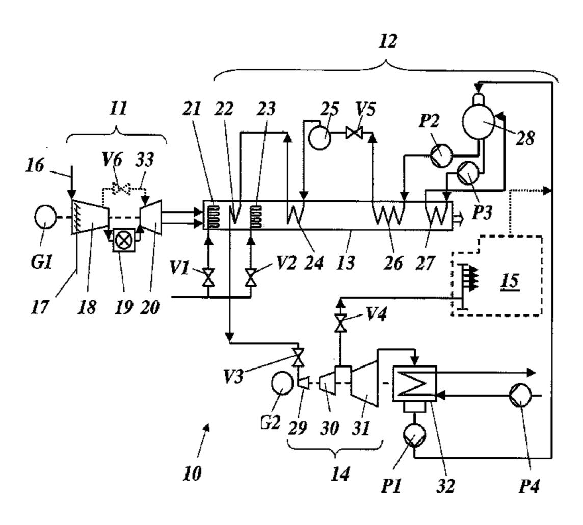
tion can be decoupled from the steam production in order to restrict the electricity production while the heat provided by steam extraction remains at a constant level. A portion of the inducted combustion air can be passed through at least one turbine to the HRSG without being involved in the combustion of the fuel in the gas turbine. This portion of the combustion air can be used to operate at least one supplementary firing in the heat recovery steam generator.
