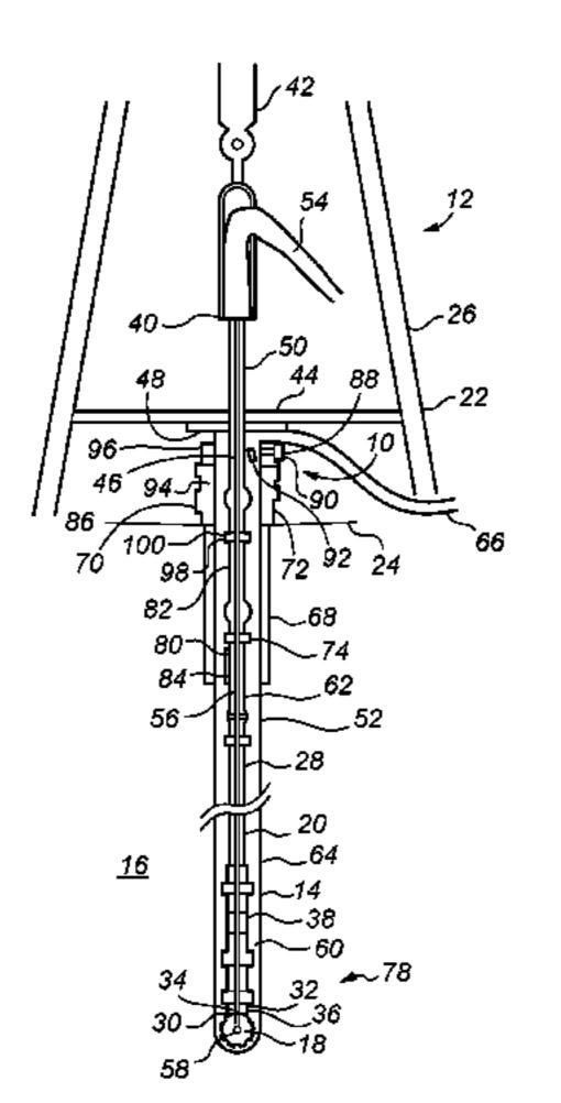
RF transmission through the wellbore using distributed RF transceivers providing data and command transmission up and down the tubing string.
